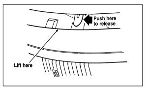
The auxiliary latch under the front edge of the hood
